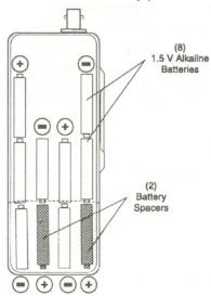
Insert the battery spacers in the positions shown so they can be easily removed.
